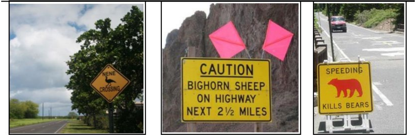
Figure 13. a) PMRF nēnē crossing sign fronting Nohili Road Curve area; b) Enhanced wildlife vehicle collision sign with flagging; c) “Red Bear, Dead Bear” sign posted at Yosemite National Park marking areas where wildlife strikes occurred along the highway
