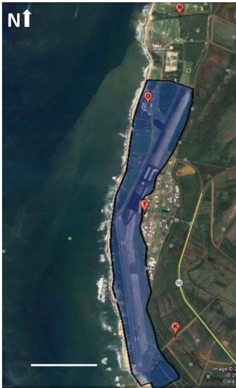
Figure 2. Nene Nest Exclusion Zone. Area of PMRF to exclude all nene nesting, generated from the lateral clear zones for the runway and taxiway.
